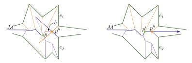
**Fig. 4.** Left: Constructing the merge chain  $\mathcal{M}$  at a specific point p where collinearities have to be handled. Right: Looking ahead lets us identify p' as start of the next horizontal bisector.
