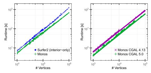
Fig. 13. Monos vs. Surfer2 on monotone inputs, and Monos with CGAL 4 vs. CGAL 5.
