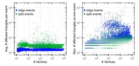
Fig. 11. Average and maximum number of triangles affected by one edge event or split event for input data of different sizes.
