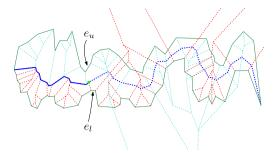
**Fig. 3.** The straight skeletons of the lower chain (dashed red) and of the upper chain (dashed turquoise). The merge (in blue) has proceeded to the point shown in green. The next bisector is defined by the edge  $e_l$  of the lower chain and the edge  $e_u$  of the upper chain.
