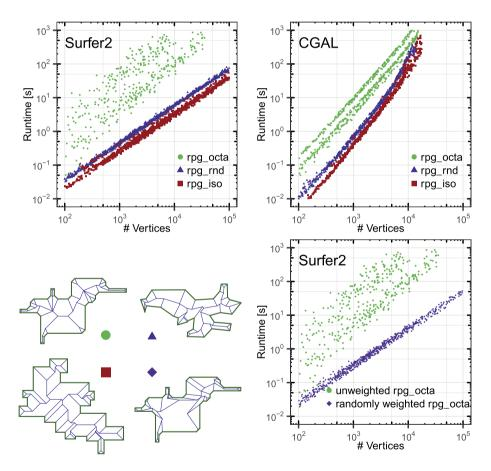
Fig. 14. Top: The effect of different input classes on the runtime of SURFER2 and on CGAL. Bottom-left: Samples for different input classes (left to right, top to bottom): Octagonal input (on integer grid), random polygon, orthogonal polygon not on integer grid, and weighted octagonal input. Bottom-right: SURFER2 runtimes for unweighted and randomly weighted octagonal input.
