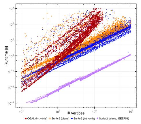
Fig. 8. Runtimes of CGAL's code and different variants of SURFER2.
